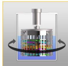
achieves a perfect infiltration of tissue, an homogeneous mixture of the reagents and a reduction of processing time. To get better results, user can start optionally a shaking process.
