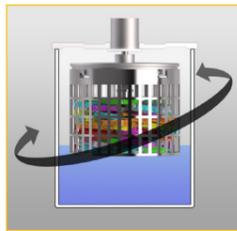
**CENTRIFUGING.** This function is activated as soon as the infiltration time comes to an end. The basket rises above the reagent's level but rests inside the vessel. For a period of 60 seconds it starts whirling at 210 rpm and changes the rotational direction every 15 seconds. This process allows tissue to be optimally drained and avoids carry-over of reagents from one vessel to another.
